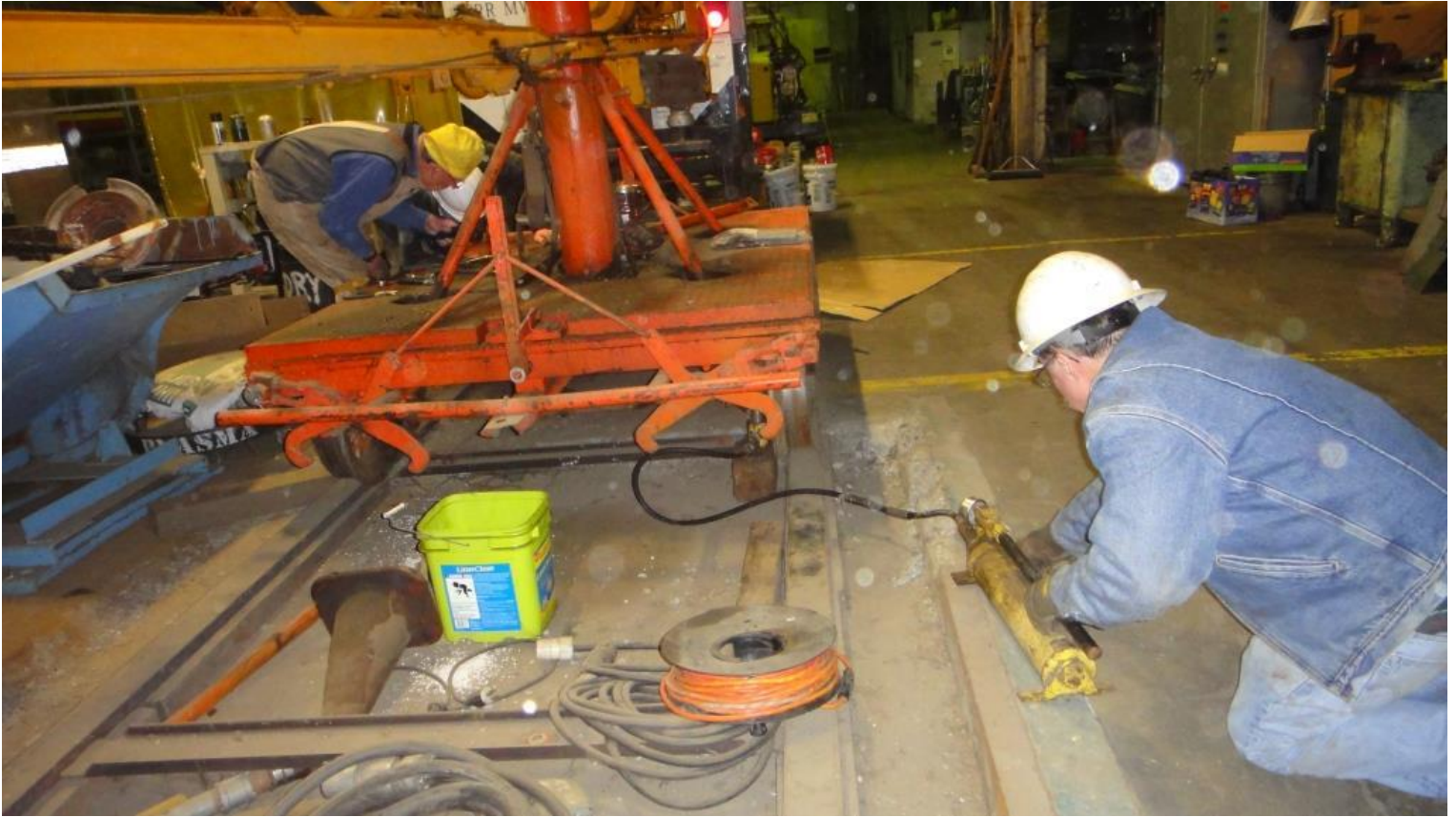
Mike H. uses a hydraulic cylinder to lift the derrick to take readings as part of his weight-measurement calculations
